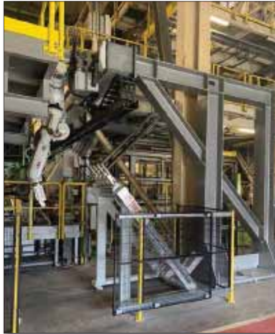
Fig 2 V-side robot on a track with the tool station
